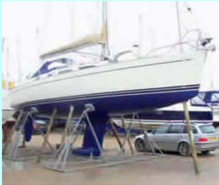
Fully adjustable Tennamast Boat-Tie yacht cradle, suitable for an up to 36ft boat of up to 7ft 2in draught
